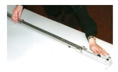
To calculate the crimp in yarn affected by knitting or weaving, to determine actual yarn usage. Threads are removed from a strip of fabrics of known length, straightened by a tension, then measured in the straightened state. Two tension ranges available (0-35 g and 0-175 g) and test length is 120 cm (48 inches).
