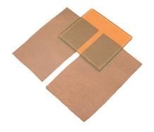
When a sample is observed to have lost color or have changed color during washing, this may be due to the effect of washing or the effect of the presence of optical brightener on the sample. This can be assessed using the fluorescence suppressor.
