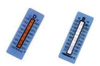
Change color to indicate maximum temperature achieved in textile processing. Self adhesive and unaffected by oil, water or steam. Ranges available from  $40^{\circ}\text{C}~(105^{\circ}\text{F})$  to  $26^{\circ}\text{C}~(500^{\circ}\text{F})$
