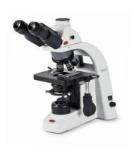
For the examination of textiles up to 1000 times magnification. Eyepieces 10x, objectives 4x, 10x, 40x, 100x, 6V / 30W quartz Halogen illumination with intensity control, 30° inclined Trinocular head with 360° rotatable head, coarse and fine focusing, vertical travel range 20 mm. Large mechanical stage with builtin X-Y verniers. Extra viewing port to cameras, video or standard.
