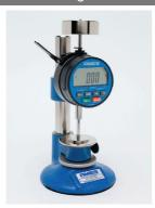
An inexpensive and accurate soft material thickness tester with counter balance designed to exert minimal load on sample through 1.129" (28.7 mm) diameter presser foot. Digital display of thickness up to 1/2" (13 mm) or 1" (25 mm). Supplied with a loading weight to provide a load of 0.6 psi (4.14 kPA). Other configurations available on application.
