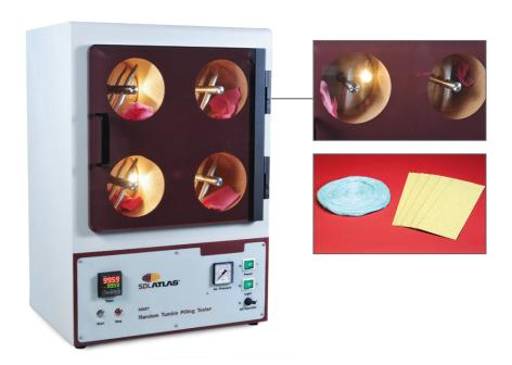
The longstanding standard instrument for ASTM D3512, the SDL Atlas Random Tumble Pilling Tester has provided consistency in pilling tests for decades. Along with the critically important cork liner, our instrument and consumables have provided confidence that results achieved today match those from when the ASTM standard was first created.
