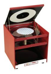
To measure and calculate the coefficient of drape by tracing a shadow of the draped fabric on paper. Supplied with three templates with paper rings with diameter of 24 cm, 30 cm and/ or 36 cm (50 pcs each).
