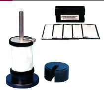
To determine a fabric's ability to recover after wrinkling under a predetermined load for a set period of time. Set of 3-D plastic replicas are available to grade fabrics.
