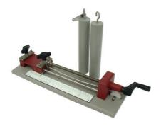
To simply and economically determine the stretch and recovery of textile fabrics, both knitted and woven. The apparatus consists of a loading frame with clamps and a screw tensioning device, two 3 kg loading weights and sample cutting templates.
