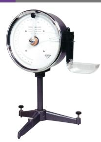
$250^{\circ}$  scale x 500 divisions. Ranges from 0-5 mg x 0.01 mg to 0-1000 mg x 2.0 mg. Also available scaled 0-500 denier for yarns (90 mm sample). Complete with pan, hook and draught excluder.
