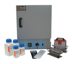
To determine colorfastness to water and perspiration of textiles. Provided with 2 stainless steel frames each with a capacity of 20 samples of 10 cm  $\times$  4 cm held between acrylic separator plates. Loading weights for BS, ISO and AATCC standards are included. An electric incubator is required available but not included.
