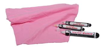
Available in fine, medium and broad ball-tips to cover all fabric types. Selection depends on the surface structure of the fabric; the finest tip used on fine, tightly woven fabric, and the broadest on open, coarse fabric. The inks are totally resistant to all textile processes indluding dry cleaning. Colors available: yellow, black, and white.
