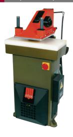
Swing arm cutting presses are ideally suited to cutting test samples from textiles, rubber and soft plastic prior to testing. Depending on resilience, several thicknesses can be cut at once with a cutting force of 20 tons. Control push buttons with time delay ensure complete operator safety. Maximum cutting area 18" (450mm) x 36" (900 mm). Cutting dies of any shape and size can be supplied.
