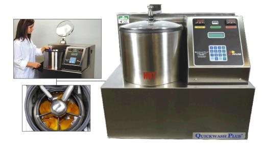
The QuickWash Plus gives fabric shrinkage information in a 12-15 minute test versus the 8-12 hours it takes a standard washer and dryer. This instrument is ideal for the factory floor and provides rapid, on the spot information on fabric in production so that the stenter frame, compactor, and sanforizer can be set to maximize fabric yield. This allows user to bypass the standard wash and dry cycles that take so long thus significantly reducing labor in the lab.
