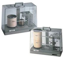
To determine and chart temperature and relative humidity over a selected period. Dual chart switchable, 1 day or 7 days with quartz clock, drive charts and pens 0-40°C, 0-90% RH.
