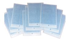
For the visual assessment and grading of Barre, the optical result of physical or dye differences in yarns, geometric differences in fabric, or a combination of both.
