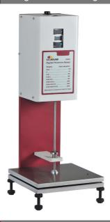
For carpet testing, with weight set 20-2000 GM/cm $^2$ , presser foot 412 mm $^2$ , range 0-25 mm x 0.01 mm.
