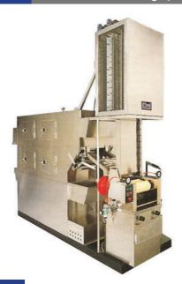
Thermosol range with infrared zone suitable for working out dye formulas and for research work.
