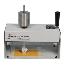
To determine the colorfastness of textiles to dry or wet rubbing particularly for printer fabrics. Applies 1134 grams of pressure on a 16 mm finger and rotates 1.125 turns clockwise then counter-clockwise. The operating handle is however turned in one direction only.
