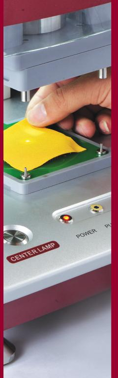
FABRIC TESTING To determine recovery properties of fabrics by creasing in a loading device for a predetermined time using a weight suitable for the test method specified (BS, ISO, AATCC). After transferring the specimen to the clamp of the tester, the specimen is allowed to recover and the angle of recovery is recorded.
