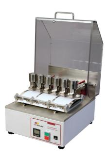
For evaluating a material's resistance to rubbing motion. Unit is a six station, benchtop machine which includes clamps for sample attachment to moving platen and clamps for weighted rubbing arm for attachment of rubbing material. Cycle counter automatically stops machine at end of test cycles. Test samples are visually evaluated.
