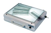
Diffused artificial daylight light source (color temperature  $5000^\circ$  K - BS 950 part 2) with 3 mm glass working surface 234 mm x 305 mm (9.2" x 12.2").
