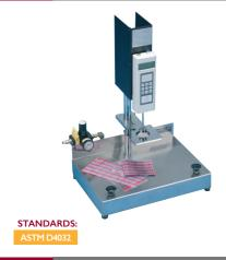
Determines fabric stiffness using the ASTM circular bend test method. A plunger of 25.4mm (1 in) diameter pushes the fabric through a 38mm (1.5 in) diameter orifice for a distance of 57mm (2.25 in) in 1.7 seconds, and the maximum force is recorded. Provided with pneumatic cylinder, controls and battery-operated digital force guage (switchable) 50 kgf / 500 N / 100 lb or 25 kgf / 250 N / 50 lb with peak-hold facility.
