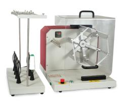
To produce skeins of yarn of a predetermined length and number of turns for count and/or strength testing. 1 Meter, 36" or 54" circumference collapsible swift (specify). Complete with yarn package stand and pretension device, fitted with predetermined counter. Available in hand operated and electronic versions.
