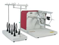
To produce skeins of yarn of a predetermined length and number of turns for count and/or strength testing. 1 meter, 36" or 54" circumference collapsible swift (specify). Complete with yarn package stand and pretension device, fitted with predetermined counter. Available in hand operated and electronic versions.
