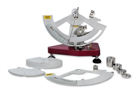
To determine the ballistic tearing strength of textiles, paper or board. Three interchangeable pendulums ranging from 8,000 to 64,000 Millinewtons (mN) can be selected seperately for multiple test method compliance.
