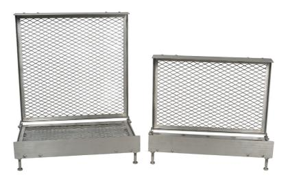
For determining the ignitability of material combinations for upholstered seating. The test rigs are covered with standard foam and fabric under test. The assembly is then ignited using one of the standard ignition sources and the combustion process is monitored.
