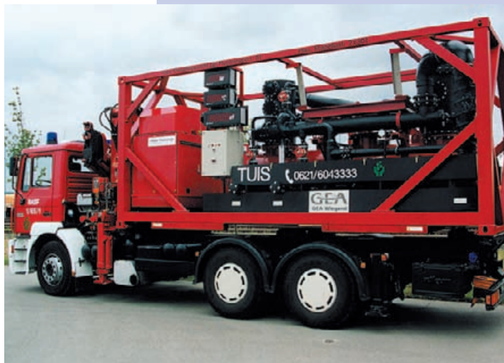
Mobile chlorine emergency unit in operation
