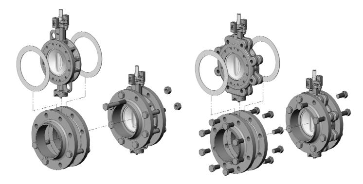
**DANGER:** When installing the butterfly valve with flanged body used in an end-of-line function, the free connection side must be additionally secured by a blind flange or (only for short-term use) the valve must be locked tightly in the "CLOSED" position. Only manual operations that are self-locking like gear operators for valves are allowed. Hand levers with notch plates do not fulfil this function!
